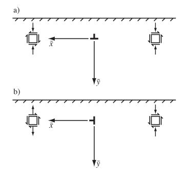
Figure 2: Elements along the  $\tilde{x}$ -axis and at symmetric points about the  $\tilde{y}$ -axis indicate stress ( $\sigma_{\tilde{x}\tilde{x}}$  omitted) due to an edge dislocation with Burgers vector a) parallel and b) perpendicular to a free surface a distance h away.
