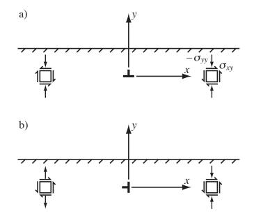
Figure 1: Elements along the x-axis and at symmetric points about the y-axis indicate stress ( $\sigma_{xx}$  omitted) due to an edge dislocation with Burgers vector a) parallel and b) perpendicular to a free surface a distance h away. Standard positive conventions for normal (in tension) and shear stresses are designated in a).
